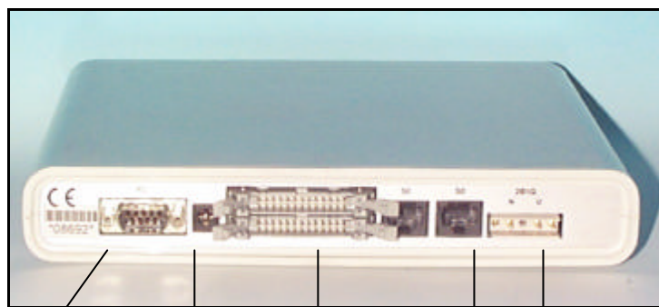
RS-232 PC/Modem Power supply Daisy Chain RJ-45 Interface S/T Connector at the U Interface
